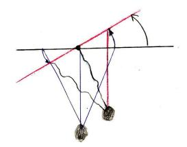
If the weight is higher than the goods, the beam rotates and the plummet will hang on one line only and the other two lines are (more or less) loose. Drawing for a EXTREME ROTATION.
