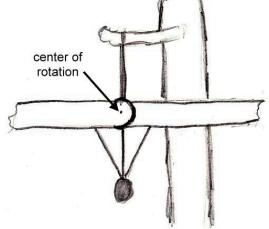
In this construction the CENTER OF ROTATION is directly over the plummet (in line with the hook).
