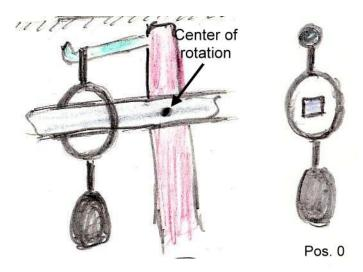
**Position 0:** The beam is free of the ring and the beam is level. Weight = goods
