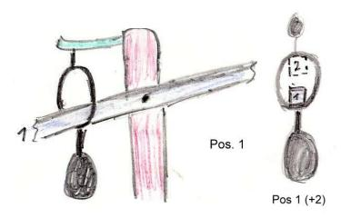
**Position 1:** If the goods are heavier than the weight, the beam touches the ring (and you can feel it on the weight)
