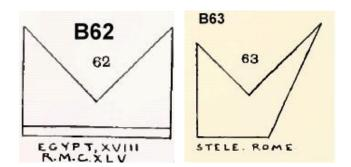
The need of a mitre square was naturally felt in Egypt; a carpenter of the xviiith dynasty has the form **62**, with a foot to slide along an edge; a bronze square with a foot, and mitre slope comes from Pompeii; and another without a foot is represented on a stele, **63**."
