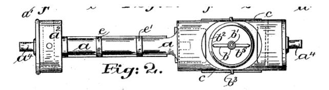
This clinometers has been principally designed to record such errors, so that the travel of a diamond drill and consequent position of the bore may from time to time be checked and charted in order to ascertain the position of the lode or other desired object as quickly and as cheaply as possible. ....
