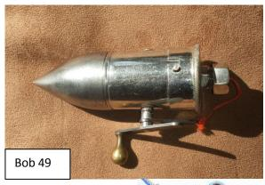
This RIDELY combination tool (chalk line and plumb bob) has a very special handle that is also used as NAIL to fix the chalk line at the beginning. So it can't get lost.
