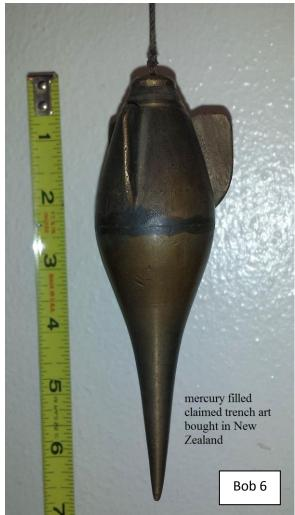
Even when this one is claimed "trench art", it may also be a modification for mining plummets, as the next drawings show. "winged plumb bobs" are used to stabilize the plumb bob in a liquid to come quicker to rest.
