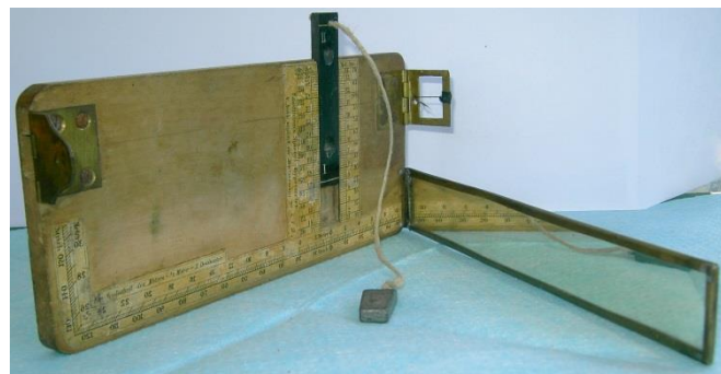
Original Faustmann hypsoneter produced by Martin Faustmann and his wife in the 1860s from my collection.
